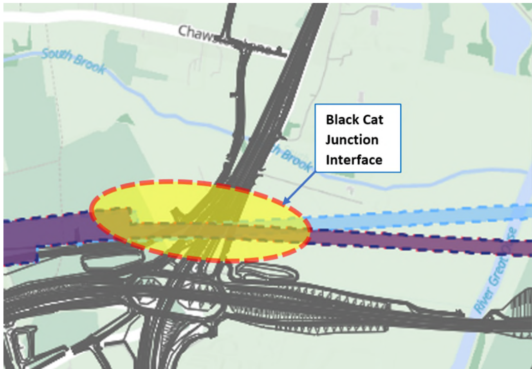
Figure 4 Potential engineering interaction location between the Scheme and EWR Project Alignments 1, 2 and 6 at the Black Cat Junction
